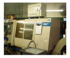
"The MistBuster 500 is a small compact unit that eats up the smoke. The units cost less and work better than other technologies."
