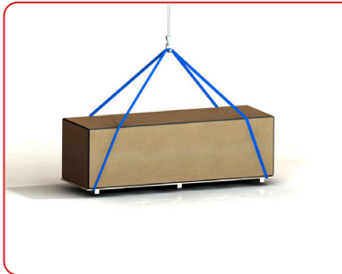
Fig.1 Use an overhead crane to lift the filter unit standing on a wooden pallet.
