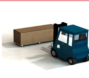
Fig. 2 Use a fork-lift to lift the filter unit standing on a wooden pallet.
