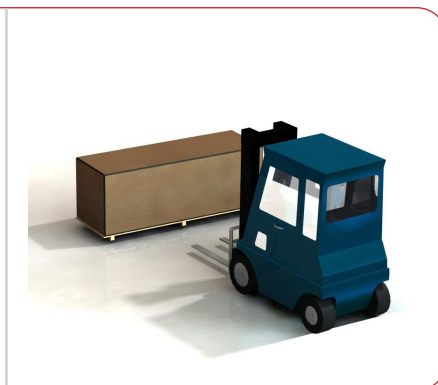
Fig. 5: Lifting the filter part and the wooden pallet with a forklift.
