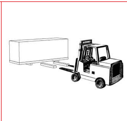
Fig.2: Lifting the filter unit on a wooden pallet with a forklift truck.
