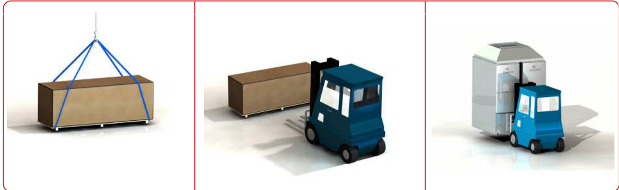
5.1.1 Lifting the filter unit on a wooden pallet with an overhead crane.
