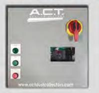
This simple all in one control provides all of the requirements needed to start and run your dust collection system. The integrated timer board and the 120V transformer allow this panel to be configured in many ways based on your needs. Below is a list of adders that can be included in this panel. All of these panels are UL Listed and can be NEMA 4 rated if your job requires the control panel to be installed outside.
