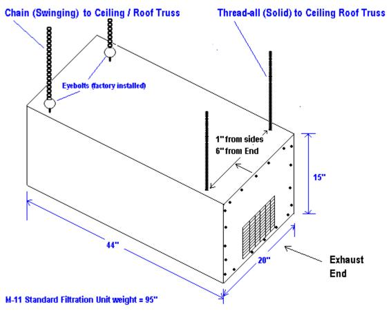
Electrical: 115VAC Single Phase with 12' power cord drawing 3.5 Amps
