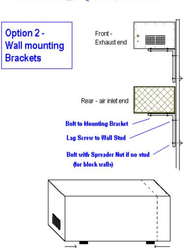
Brackets under cabinet installed 6" in from ends or 32" on centers (lines up with wall studs)
